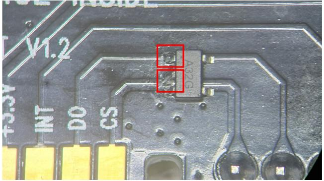
Then solder in the SN74AHC1G32 pin 1 and 2 on DO and CS on the tinned side.
