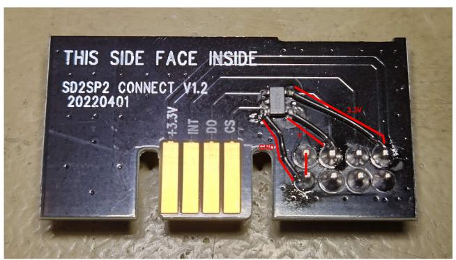
Then solder from SN74AHC1G32 pin 3 to GND, pin 5 to 3.3V, pin 4 to Y (old DO), and the last step is bridging GND and old CS.
