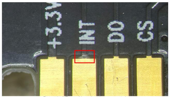
First cut the INT trace, this one is no longer connected.
