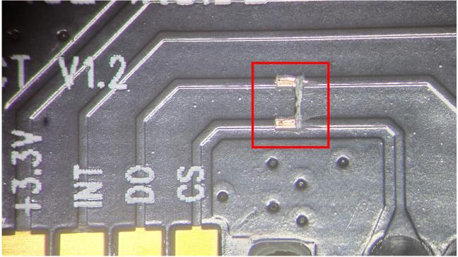
Then cut the DO and CS trace, scrape and tin the traces from those on the side going to the edge connector.
